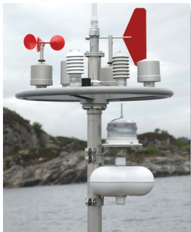
*The Mast Section is equipped with a Mini Tri-Lens Reflector (The reflector coverage is 330 degrees) and a Sealite Flashing Light, SL 15.*
