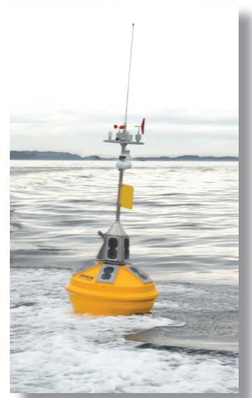
*The Buoy is cone-shaped with a low centre of gravity; this provides High Stability and reduces wear and tear of Cables.*
