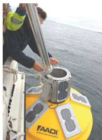
*The buoy is of modular design which enables a variety of applications.*
